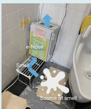
Fig. 8 Odor experimental measurement in a restroom
